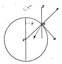
$\omega$  be the angular velocity of the earth, b the distance of the point O from the axis of rotation.
